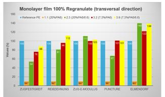
Fig. 5b: Mechanical film properties, dilution without compatibilizer (transversal)
