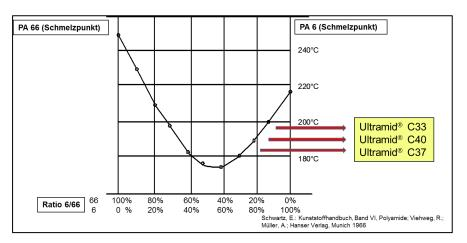
Fig. 35: Correlation of melting points of PA6/6.6 copolyamides
