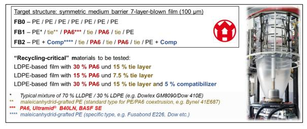
Fig. 24: Overview of test structures for PE/PA6 program section (Ultramid<sup>®</sup> B40LN)
