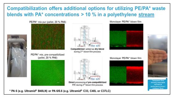
Fig. 21: Summary of process recommendation for PE/PA mixtures with >/= 10 % PA
