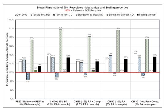
Fig. 34: Mechanical characteristic values of various recyclate samples, measured on the basis of blown films
