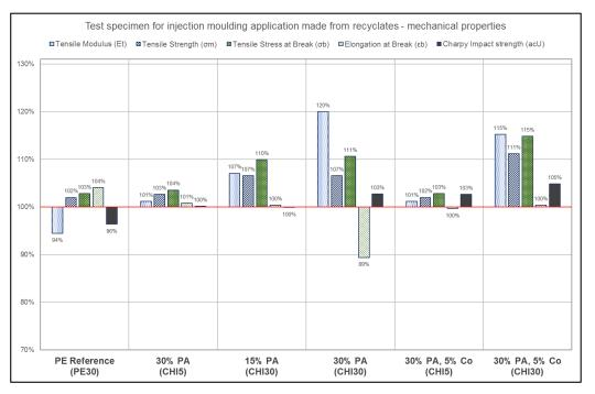
Fig. 28: Mechanical characteristic values of various recyclate samples, measured on the basis of injection molding specimens
