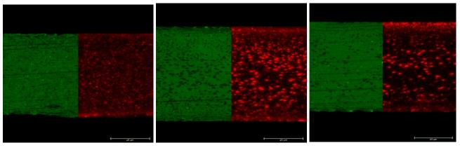
Fig. 10: Morphology of film 4.10 (contains 15 % PA6/6.6 and 3 % E226)
