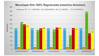
Fig. 5a: Mechanical film properties, dilution without compatibilizer (longitudinal)
