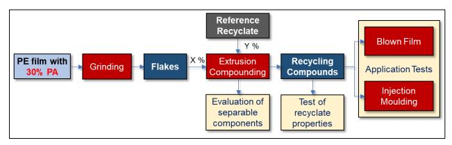
Fig. 23: Schematic diagram of the CHI standard test method CHI-C8-PEF-1
