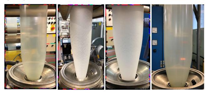
Fig. 29a–d: Visual appearance of the monofilm bubble (melt temperature): a) 5 % PA6 (215°C) b) 15 % PA6 (215°C) c) 15 % PA6 (235°C) d) 0.75 % PA6/6.6 (210°C)
