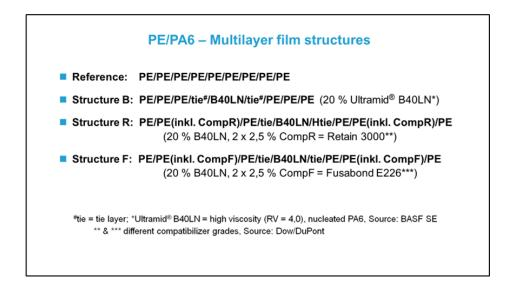
Fig. 2: Selected examples of multilayer film structures investigated
