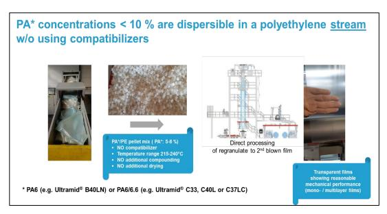
Fig. 20: Summary of process recommendation for PE/PA mixtures with < 10 % PA
